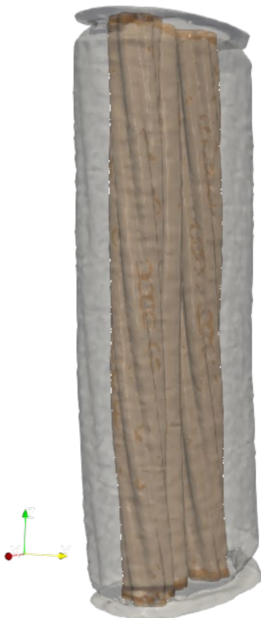
Fig. 3: Visualisation of the 3D model of the electric cable. Transparency is used to show the copper wires inside the insulating material.
